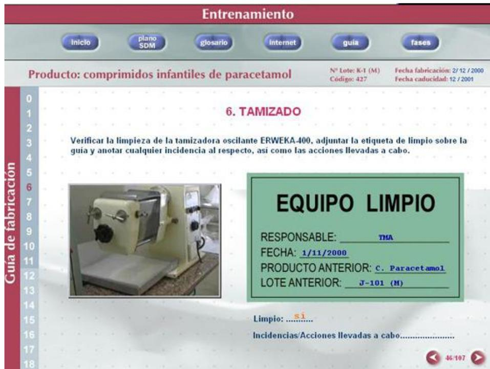
Figure 4. Part III. Training. Third part of the application: Training for tablet manufacturing. Example of a screenshot showing the label to be used in the laboratory after cleaning the sieving machine.
